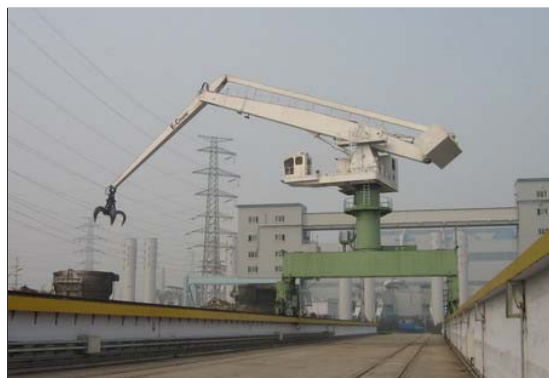
TISCO E-Crane® nr. 1, gantry-based on rail, sorting scrap and filling baskets at Taiyuan scrap yard.
